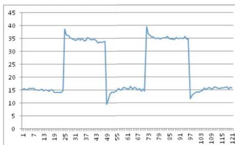
The above plot shows the resulting transient temperature changes in a reactor equipped to perform power compensated calorimetry. The 4547 jacketed reactor used here has an internal volume of 1.2 L and was half full of water. Data were recorded at one minute intervals while the set point bias was toggled 1.5 C. The y-axis is the trim heater power (watts).
