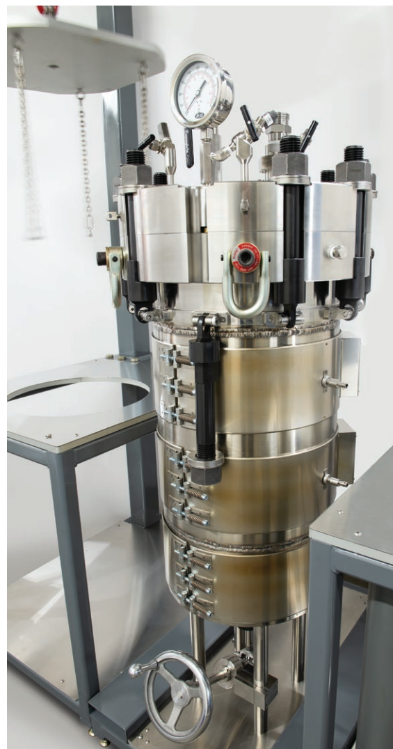
100 L vessel with one Qik-Latch Bolt open
