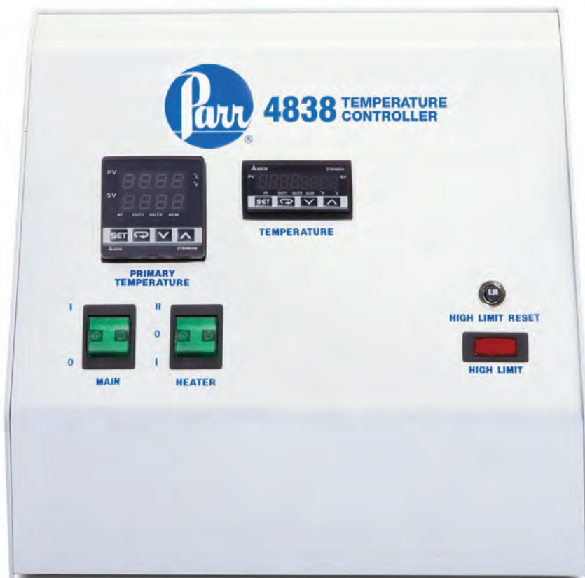
Parr 4838 Reactor Controller shown with optional HTM Module
