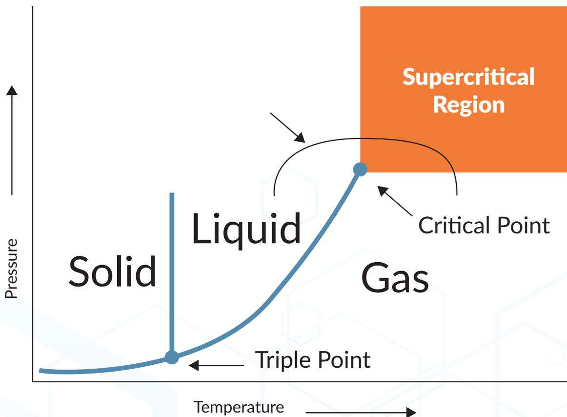
Figure 1-1: Supercritical CO<sub>2</sub> is tuneable without changing phases
