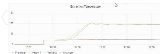
Building on our pressure control, the SFX Software has a built-in temperature ramp feature, allowing the user to control the rate of heating.
