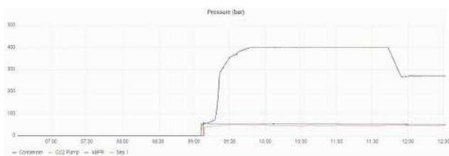
Depressurisation control on many other control systems simply involves the controlled opening of the BPR needle over time. The user calibrates the needle speed to achieve the necessary setpoint. The SFX software removes this trial and error and introduces true depressurisation control through a ramp rate setpoint and pressure control feedback.
