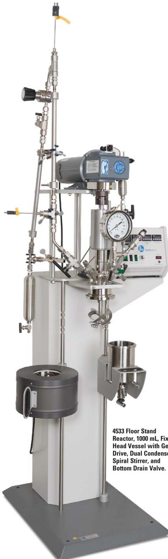
4533 Floor Stand Reactor, 1000 mL, Fixed Head Vessel with Gear Drive, Dual Condenser, Spiral Stirrer, and Bottom Drain Valve.
