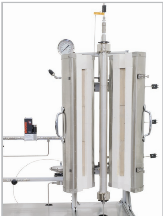
Open 3-zone Split Tube Furnace with 1" I.D. Tubular Reactor.
