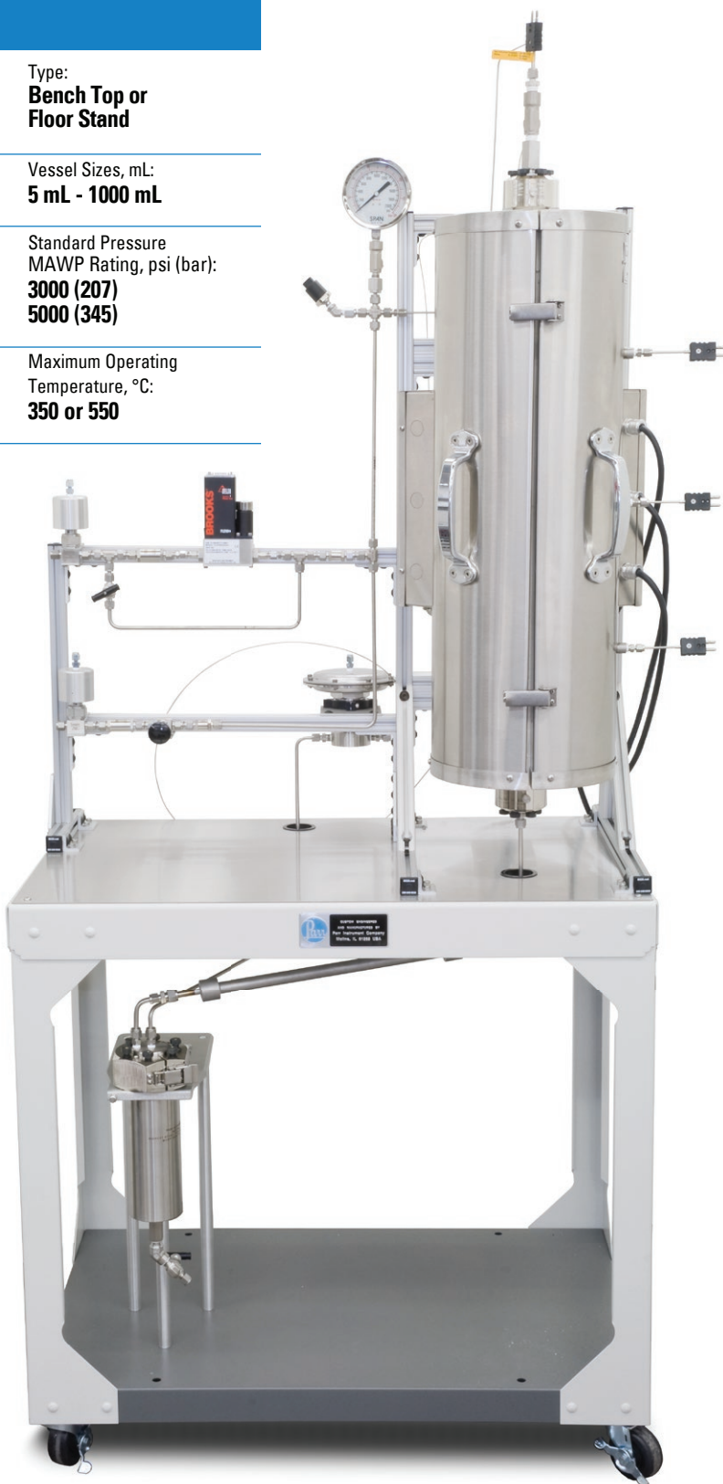
Model 5403 with a 1" inside dia. x 24" length, 3-zone split tube furnace with gas feed system, cooling condenser, gas/liquid separator vessel and automated back pressure regulator.
