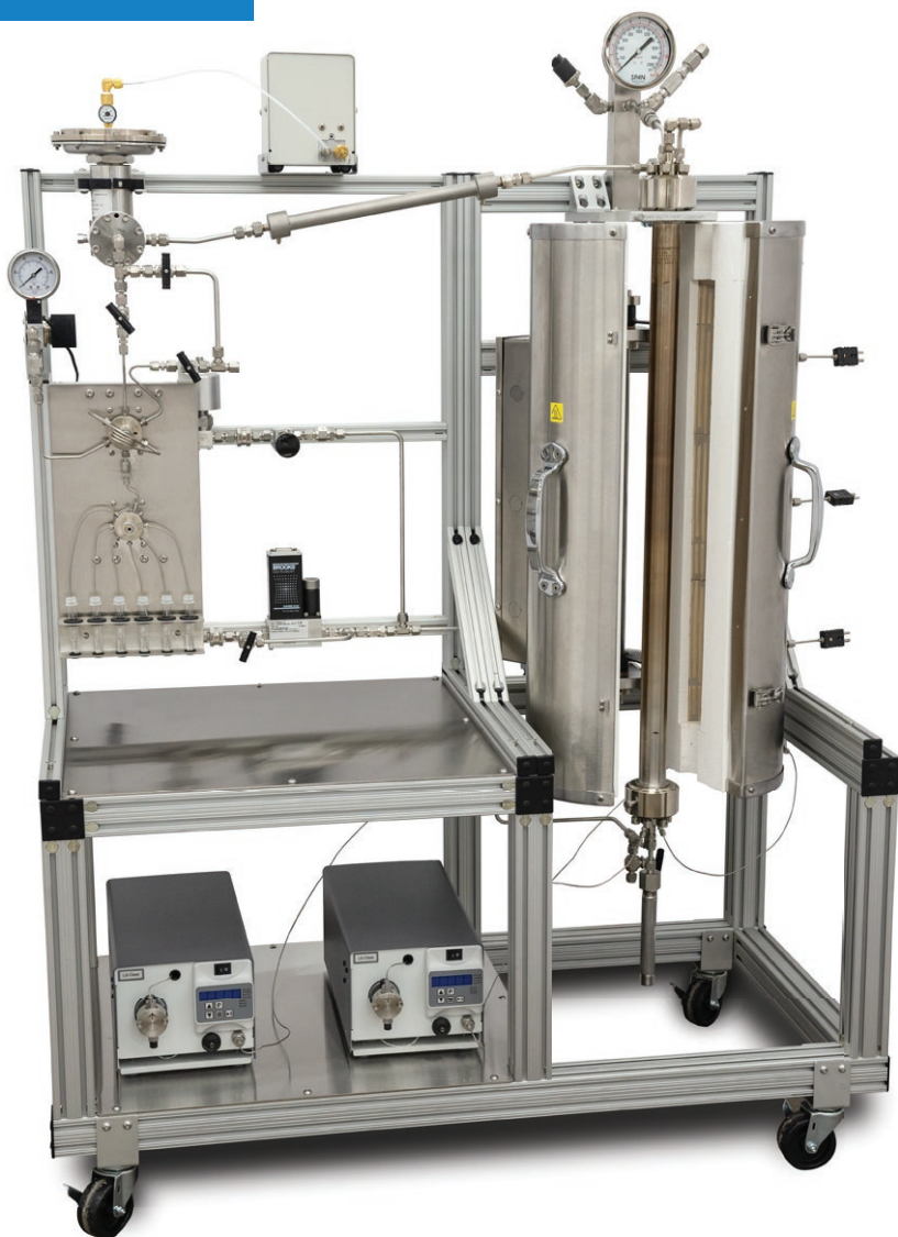
Up-flow 5403 Tubular Reactor System with 300 mL heated volume, one purge line, one gas feed, two liquid feeds, product cooling condenser, and automated 2-phase back pressure regulator. An automated liquid sampler captures representative samples at user-programmable intervals.
