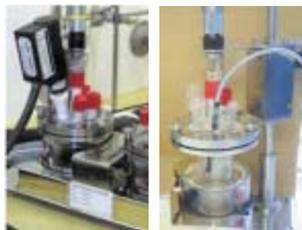
A Lasentec probe within an HEL auto-MATE reactor
