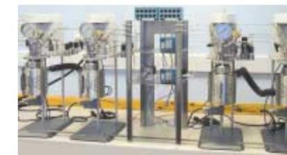
400ml system customised with gas and liquid feeds
