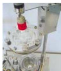
Enzymatic reactor with replaceable sinter and automatic valve in base
