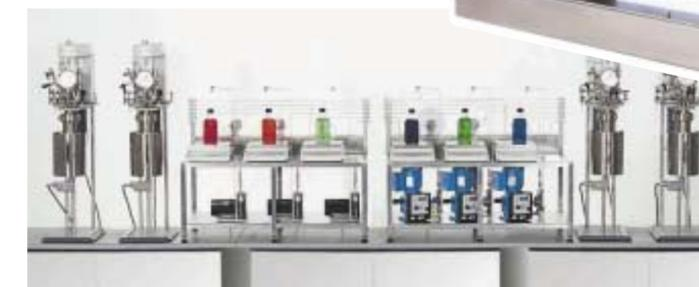
400ml system with 6 high pressure independent feeds to all 4 vessels
