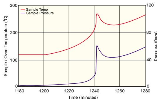
Thermal screening of a nitrocellulose dye at 2°C/min from ambient to 280°C
