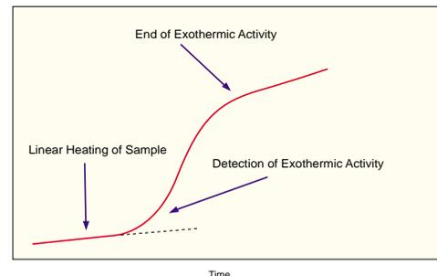
Linear ramp of sample – deviation from linearity indicates exotherm
