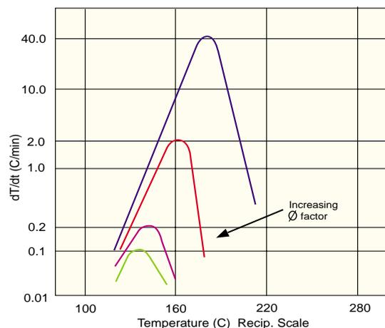
Rate of temperature rise using different test cells
