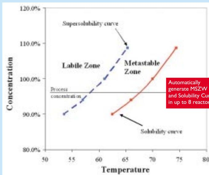
Automatic sequential dosing with 1, 2, or more solvents to automatically generate solubility and metastable zone data.
