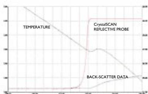
*Turbidity mode used in CrystalSCAN: The reflectance technique, suitably optimised, gives earlier and reliable detection of solids - also more sensitive than human eye.*
