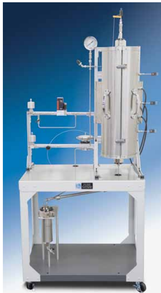
Model 5403 with a 1" inside dia. x 24" length, 3-zone clam shell heater with gas & liquid feed system.
