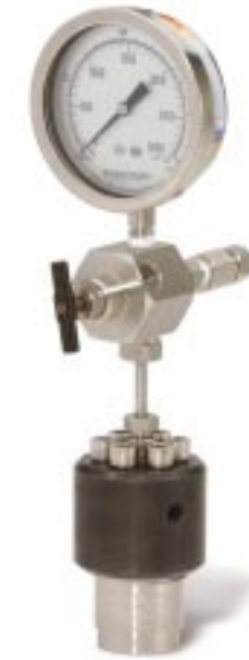
Model 4742, 25 mL Vessel, with Gage Block Assembly
