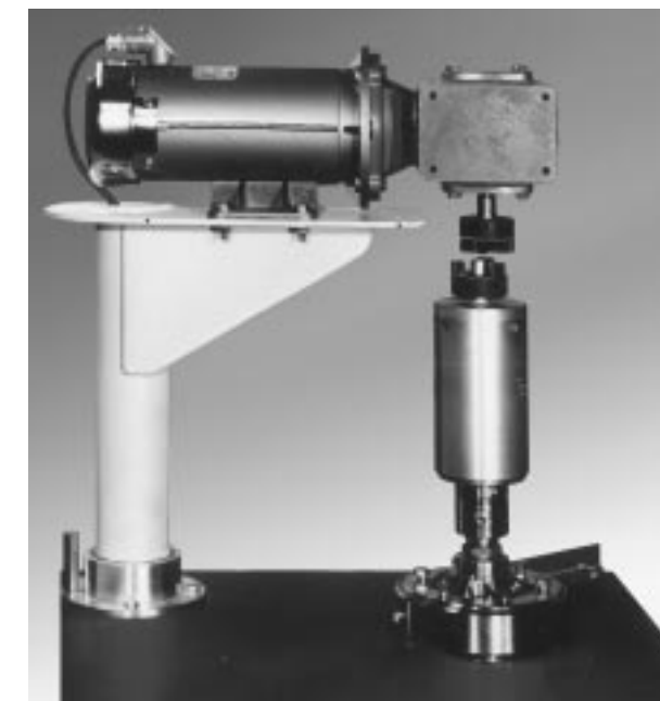
Geared Drive Motor with Cover Removed
