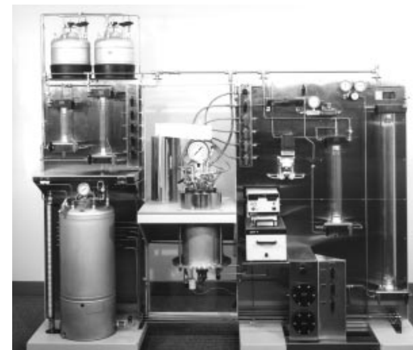
Custom Built Catalyst Preparation System
