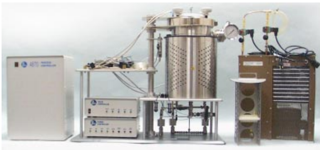
Custom Turn-Key System with 4870 Process Controller, Custom Power and Valve Controllers, Automated Valving/Interlock/Cooling Systems
